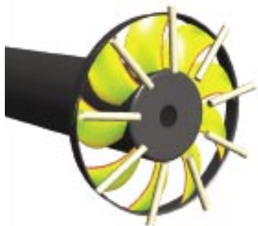
Unsteady forces on fan blades generating noise
