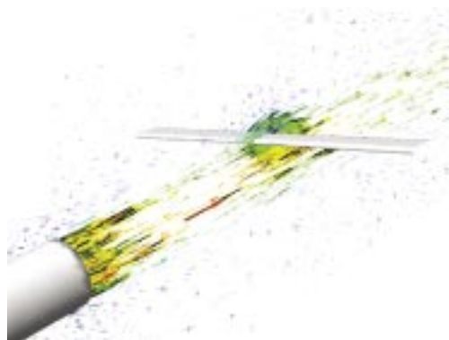
Noise from a strut present in a turbulent subsonic jet
